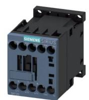
power contactor, AC-3e/AC-3, 12 A, 5.5 kW / 400 V, 3-pole, 200 V AC, 50 Hz / 200-220 V, 60 Hz, auxiliary contacts: 1 NC, screw terminal, size: S00
