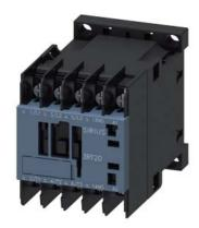
power contactor, AC-3e/AC-3, 9 A, 4 kW / 400 V, 3-pole, 220 V AC, 50 Hz / 240 V, 60 Hz, auxiliary contacts: 1 NO, ring cable lug connection, size: S00
