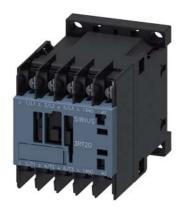
power contactor, AC-3e/AC-3, 9 A, 4 kW / 400 V, 3-pole, 200 V AC, 50 Hz / 200-220 V, 60 Hz, auxiliary contacts: 1 NO, ring cable lug connection, size: S00
