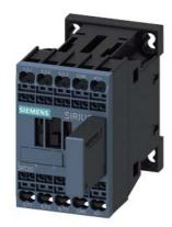
power contactor, AC-3e/AC-3, 9 A, 4 kW / 400 V, 3-pole, 24 V DC, 0.85-1.85\* Us, with varistor plugged on, auxiliary contacts: 1 NC, spring-loaded terminal, size: S00, not expandable with auxiliary switch
