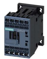
power contactor, AC-3e/AC-3, 9 A, 4 kW / 400 V, 3-pole, 24 V DC, 0.85-1.85\* Us, with integrated suppressor diode, auxiliary contacts: 1 NC, spring-loaded terminal, size: S00
