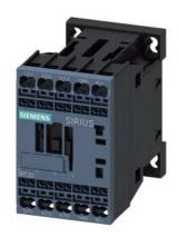
power contactor, AC-3e/AC-3, 9 A, 4 kW / 400 V, 3-pole, 24 V DC, 0.85-1.85\* Us, auxiliary contacts: 1 NO, spring-loaded terminal, size: S00, not expandable with auxiliary switch
