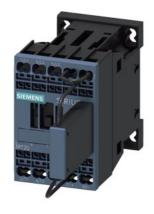
traction contactor, AC-3e/AC-3, 9 A, 4 kW / 400 V, 3-pole, 72 V DC, 0.7-1.25 $^{\star}$  Us, with integrated varistor, auxiliary contacts: 1 NC, spring-loaded terminal, size: S00, with plugged on series resistor
