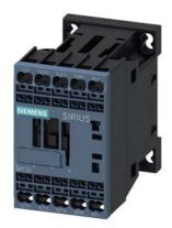
power contactor, AC-3e/AC-3, 9 A, 4 kW / 400 V, 3-pole, 24 V DC, 0.7-1.25 $^{\star}$  Us, with integrated diode, auxiliary contacts: 1 NC, spring-loaded terminal, size: S00, suitable for PLC outputs, not expandable with auxiliary switch
