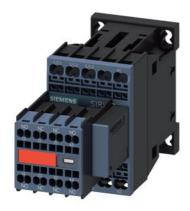
power contactor, AC-3e/AC-3, 9 A, 4 kW / 400 V, 3-pole, 230 V AC, 50/60 Hz, with varistor plugged on, auxiliary contacts: 2 NO + 2 NC, spring-loaded terminal, size: S00, captive auxiliary switch
