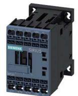
power contactor, AC-3e/AC-3, 9 A, 4 kW / 400 V, 3-pole, 230 V AC, 50/60 Hz, auxiliary contacts: 1 NO, spring-loaded terminal, size: S00
