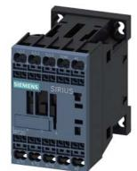
power contactor, AC-3e/AC-3, 9 A, 4 kW / 400 V, 3-pole, 220 V AC, 50/60 Hz, auxiliary contacts: 1 NC, spring-loaded terminal, size: S00
