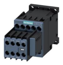
power contactor, AC-3e/AC-3, 9 A, 4 kW / 400 V, 3-pole, 120 V AC, 50/60 Hz, with varistor plugged on, auxiliary contacts: 3 NO + 2 NC, screw terminal, size: S00, removable auxiliary switch
