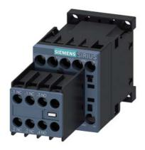
power contactor, AC-3e/AC-3, 9 A, 4 kW / 400 V, 3-pole, 24 V DC, auxiliary contacts: 1 NC, screw terminal, size: S00, removable auxiliary switch
