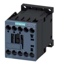
power contactor, AC-3e/AC-3, 9 A, 4 kW / 400 V, 3-pole, 24 V DC, auxiliary contacts: 1 NO, screw terminal, size: S00, communication-capable
