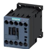
power contactor, AC-3e/AC-3, 9 A, 4 kW / 400 V, 3-pole, 200 V AC, 50 Hz / 200-220 V, 60 Hz, auxiliary contacts: 1 NC, screw terminal, size: S00
