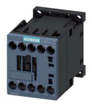
power contactor, AC-3e/AC-3, 9 A, 4 kW / 400 V, 3-pole, 110 V AC, 50/60 Hz, auxiliary contacts: 1 NO, screw terminal, size: S00, upright mounting position
