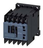
power contactor, AC-3e/AC-3, 7 A, 3 kW / 400 V, 3-pole, 220 V AC, 50 Hz / 240 V, 60 Hz, auxiliary contacts: 1 NC, ring cable lug connection, size: S00
