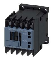
power contactor, AC-3e/AC-3, 7 A, 3 kW / 400 V, 3-pole, 200 V AC, 50 Hz / 200-220 V, 60 Hz, auxiliary contacts: 1 NO, ring cable lug connection, size: S00
