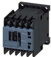
power contactor, AC-3e/AC-3, 7 A, 3 kW / 400 V, 3-pole, 110 V AC, 50 Hz / 120 V, 60 Hz, auxiliary contacts: 1 NC, ring cable lug connection, size: S00  $\,$
