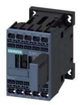
power contactor, AC-3e/AC-3, 7 A, 3 kW / 400 V, 3-pole, 24 V DC, 0.7-1.25\* Us, with varistor plugged on, auxiliary contacts: 1 NC, spring-loaded terminal, size: S00, not expandable with auxiliary switch
