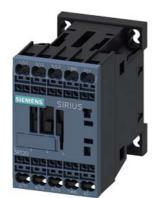
power contactor, AC-3e/AC-3, 7 A, 3 kW / 400 V, 3-pole, 48 V DC, auxiliary contacts: 1 NO, spring-loaded terminal, size: S00,
