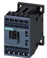
power contactor, AC-3e/AC-3, 7 A, 3 kW / 400 V, 3-pole, 220 V DC, auxiliary contacts: 1 NO, spring-loaded terminal, size: S00,
