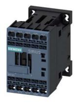
power contactor, AC-3e/AC-3, 7 A, 3 kW / 400 V, 3-pole, 110 V DC, auxiliary contacts: 1 NC, spring-loaded terminal, size: S00,
