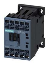
power contactor, AC-3e/AC-3, 7 A, 3 kW / 400 V, 3-pole, 60 V DC, auxiliary contacts: 1 NC, spring-loaded terminal, size: S00,
