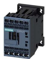
power contactor, AC-3e/AC-3, 7 A, 3 kW / 400 V, 3-pole, 24 V DC, auxiliary contacts: 1 NC, spring-loaded terminal, size: S00, upright mounting position
