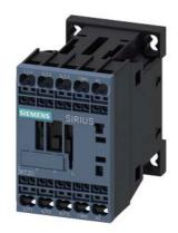
power contactor, AC-3e/AC-3, 7 A, 3 kW / 400 V, 3-pole, 400 V AC, 50/60 Hz, auxiliary contacts: 1 NO, spring-loaded terminal, size: S00,
