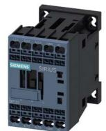
power contactor, AC-3e/AC-3, 7 A, 3 kW / 400 V, 3-pole, 220 V AC, 50/60 Hz, auxiliary contacts: 1 NO, spring-loaded terminal, size: S00,
