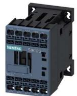
power contactor, AC-3e/AC-3, 7 A, 3 kW / 400 V, 3-pole, 48 V AC, 50/60 Hz, auxiliary contacts: 1 NO, spring-loaded terminal, size: S00,
