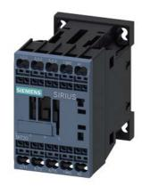
power contactor, AC-3e/AC-3, 7 A, 3 kW / 400 V, 3-pole, 42 V AC, 50/60 Hz, auxiliary contacts: 1 NO, spring-loaded terminal, size: S00,
