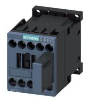
power contactor, AC-3e/AC-3, 7 A, 3 kW / 400 V, 3-pole, 24 V DC, 0.7-1.25\* Us, with varistor plugged on, auxiliary contacts: 1 NO, screw terminal, size: S00, not expandable with auxiliary switch
