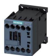
power contactor, AC-3e/AC-3, 7 A, 3 kW / 400 V, 3-pole, 24 V DC, 0.85-1.85\* Us, auxiliary contacts: 1 NO, screw terminal, size: S00, not expandable with auxiliary switch
