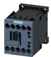
power contactor, AC-3e/AC-3, 7 A, 3 kW / 400 V, 3-pole, 24 V DC, 0.7-1.25\* Us, auxiliary contacts: 1 NC, screw terminal, size: S00, suitable for PLC outputs, not expandable with auxiliary switch
