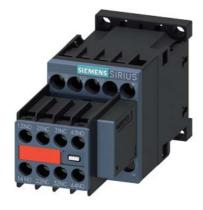
power contactor, AC-3e/AC-3, 7 A, 3 kW / 400 V, 3-pole, 230 V AC, 50/60 Hz, with varistor plugged on, auxiliary contacts: 2 NO + 2 NC, screw terminal, size: S00, captive auxiliary switch
