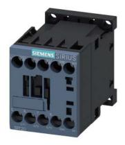
power contactor, AC-3e/AC-3, 7 A, 3 kW / 400 V, 3-pole, 230 V DC, auxiliary contacts: 1 NC, screw terminal, size: S00,
