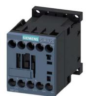
power contactor, AC-3e/AC-3, 7 A, 3 kW / 400 V, 3-pole, 24 V DC, auxiliary contacts: 1 NC, screw terminal, size: S00, upright mounting position
