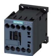
power contactor, AC-3e/AC-3, 7 A, 3 kW / 400 V, 3-pole, 110 V AC, 50 Hz / 120 V, 60 Hz, auxiliary contacts: 1 NO, screw terminal, size: S00, upright mounting position
