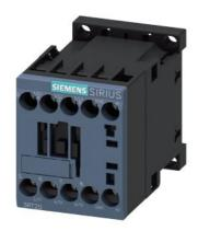
power contactor, AC-3e/AC-3, 7 A, 3 kW / 400 V, 3-pole, 24 V AC, 50/60 Hz, auxiliary contacts: 1 NC, screw terminal, size: S00, upright mounting position
