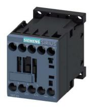
power contactor, AC-3e/AC-3, 7 A, 3 kW / 400 V, 3-pole, 24 V AC, 50/60 Hz, auxiliary contacts: 1 NO, screw terminal, size: S00, upright mounting position
