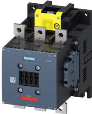
power contactor AC-1 400 A / 690 V / 40 °C 3-pole, U<sub>c</sub>: 96-127 V AC(50-60 Hz) / DC F-PLC input 24 V DC drive: electronic auxiliary contacts 2 NO + 2 NC main circuit: busbar control and auxiliary circuit: screw terminal
