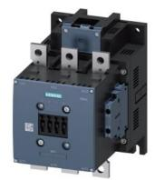
power contactor AC-1 400 A / 690 V / 40 °C 3-pole, Uc: 200-277 V AC(50-60 Hz) / DC PLC input 24 V DC drive: electronic auxiliary contacts 2 NO + 2 NC main circuit: busbar control and auxiliary circuit: screw terminal
