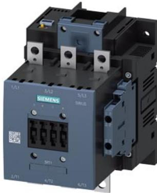
power contactor AC-1 275 A / 690 V / 40 °C 3-pole, U<sub>c</sub>: 96-127 V AC(50-60 Hz) / DC PLC input 24 V DC drive: electronic auxiliary contacts 2 NO + 2 NC main circuit: busbar control and auxiliary circuit: screw terminal
