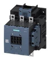
power contactor AC-1 275 A / 690 V / 40  $^{\circ}$ C 3-pole, Uc: 380-420 V AC(50-60 Hz) / DC drive: conventional auxiliary contacts 2 NO + 2 NC main circuit: busbar control and auxiliary circuit: screw terminal
