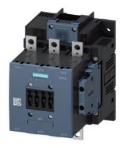
power contactor AC-1 275 A / 690 V / 40  $^{\circ}$ C 3-pole, Uc: 500-550 V AC(50-60 Hz) / DC drive: conventional auxiliary contacts 2 NO + 2 NC main circuit: busbar control and auxiliary circuit: screw terminal
