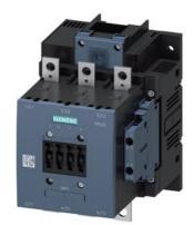
power contactor AC-1 275 A / 690 V / 40  $^\circ$ C 3-pole, Uc: 200-220 V AC(50-60 Hz) / DC drive: conventional auxiliary contacts 2 NO + 2 NC main circuit: busbar control and auxiliary circuit: screw terminal
