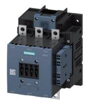
power contactor AC-1 275 A / 690 V / 40  $^\circ$ C 3-pole, Uc: 23-26 V AC(50-60 Hz) / DC drive: conventional auxiliary contacts 2 NO + 2 NC main circuit: busbar control and auxiliary circuit: screw terminal
