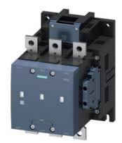
vacuum contactor AC-3e/AC-3 265 A, 132 kW / 400 V, 3-pole, Uc: 440-480 V AC(50-60 Hz) / DC drive: conventional auxiliary contacts 2 NO + 2 NC main circuit: busbar control and auxiliary circuit: screw terminal
