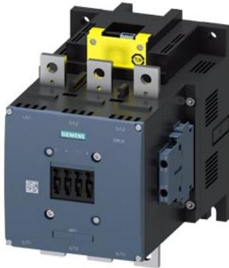
power contactor, AC-3e/AC-3 400 A, 200 kW / 400 V AC (50-60 Hz) / DC 200-277 V x (0.8-1.1) F-PLC input 24 V DC 3-pole, auxiliary contacts 2 NO + 2 NC drive: electronic main circuit: busbar control and auxiliary circuit: screw terminal
