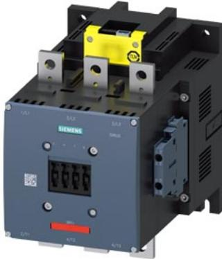
power contactor, AC-3e/AC-3 400 A, 200 kW / 400 V AC (50-60 Hz) / DC 96-127 V x (0.8-1.1) F-PLC input 24 V DC 3-pole, auxiliary contacts 2 NO + 2 NC
