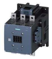
power contactor, AC-3e/AC-3 400 A, 200 kW / 400 V AC (50-60 Hz) / DC Uc: 575-600 V 3-pole, auxiliary contacts 2 NO + 2 NC drive: conventional main circuit: busbar control and auxiliary circuit: screw terminal
