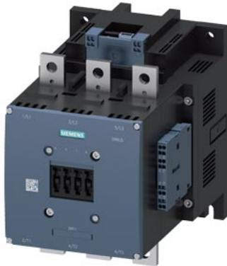
power contactor, AC-3e/AC-3 400 A, 200 kW / 400 V U<sub>c</sub>: 72 V DC x (0.7-1.25) PLC input 24-110 V DC 3-pole, auxiliary contacts 2 NO + 2 NC drive: electronic main circuit: busbar control and auxiliary circuit: spring-loaded terminal extended rated condition railroad IEC 60077
